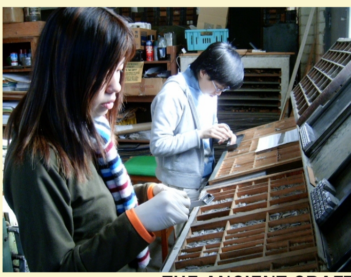
THE ANCIENT CRAFT OF TYPESETTING BY HAND IS PRACTICED AND PASSED ON MECHANICAL TYPESETTING MACHINE (LINTYPE) AND ITS OUTPUT THEY LEARN BETTER BY HAND
